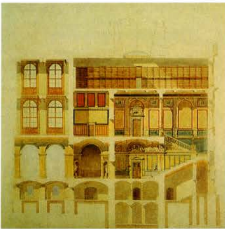
Cross-section of the library wing of Vienna University. Coloured pen-and-ink drawing by Heinrich Ferstel, signed and dated 1877.
