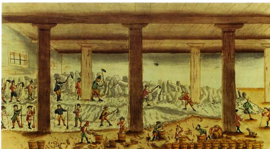
Salt production in the Salzkammergut: depiction from ca. 1656 of “Fuderhacken und Küferstossen”, showing how the blocks of salt were broken up and crushed and then put into wooden barrels for transportation.
